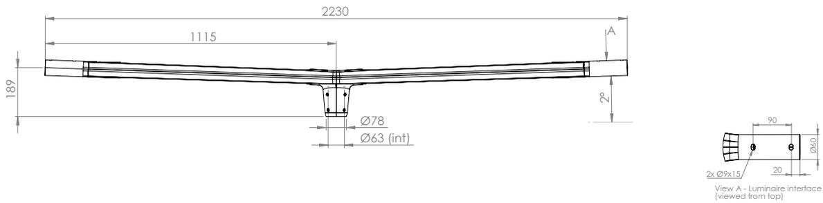
KEMA top double penetrating on pole Ø76
