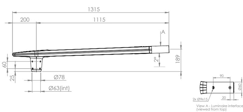
KEMA top simple penetrating on pole Ø76
