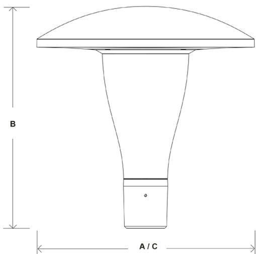
PILZEO | Fixation enveloppante Ø60 mm - 2 vis M8
